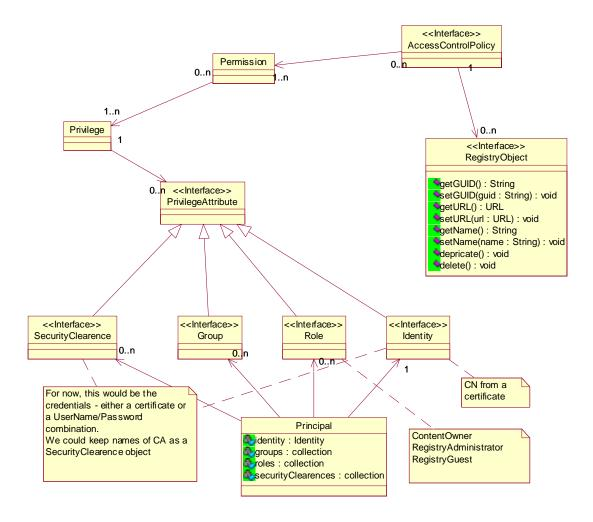
The AccessControlPolicy is the top-level security object. It ties together the permission object with an instance of a Registry object. The permission object also contains the methods (of the RegistryObject), which the privilege object can access.
