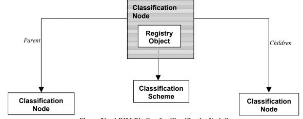
Figure 21: ebRIM Binding for ClassificationNodeQuery
