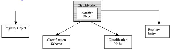
Figure 20: ebRIM Binding for ClassificationQuery
