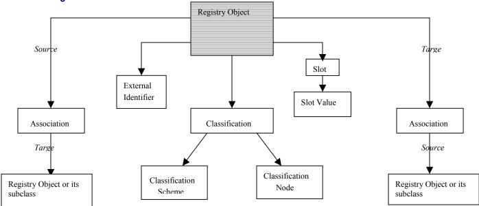
Figure 16: ebRIM Binding for RegistryObjectQuery
