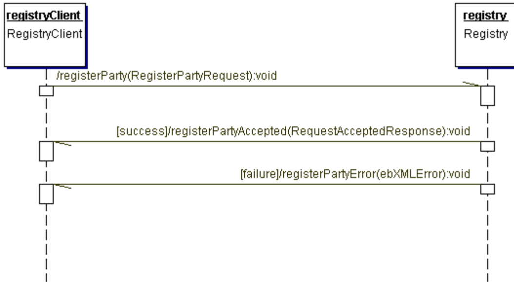
Figure 2: Bootstrap Registration Process Sequence Diagram
