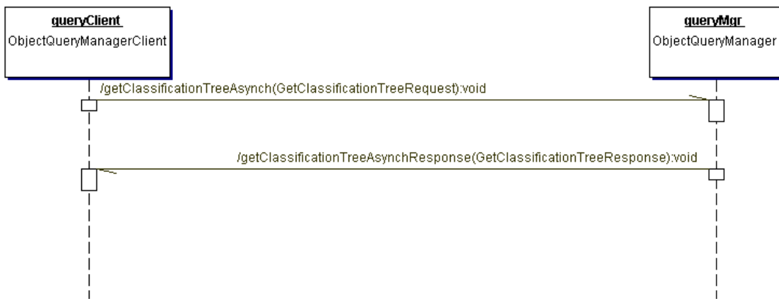
561 Figure 11: Get Classification Tree Asynchronous Sequence Diagram
