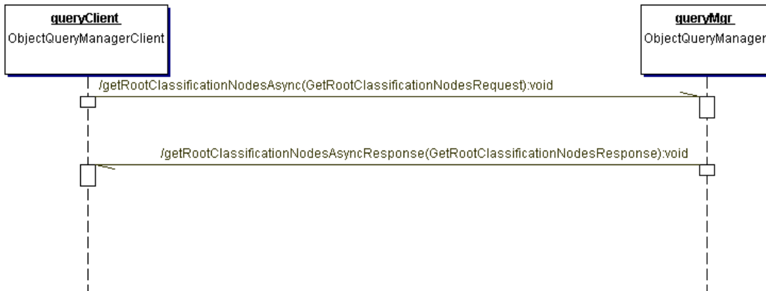
Figure 8: Get Root Classification Nodes Sequence Diagram
