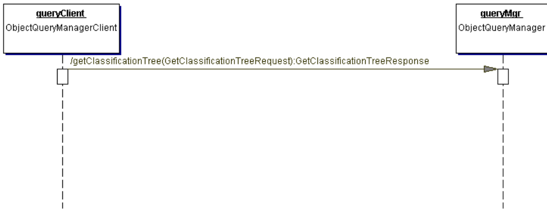
559 Figure 10: Get Classification Tree Sequence Diagram
