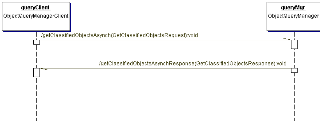
Figure 13: Get Classified Objects Asynchronous Sequence Diagram
