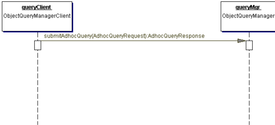
Figure 16: Submit Ad Hoc Query Sequence Diagram
