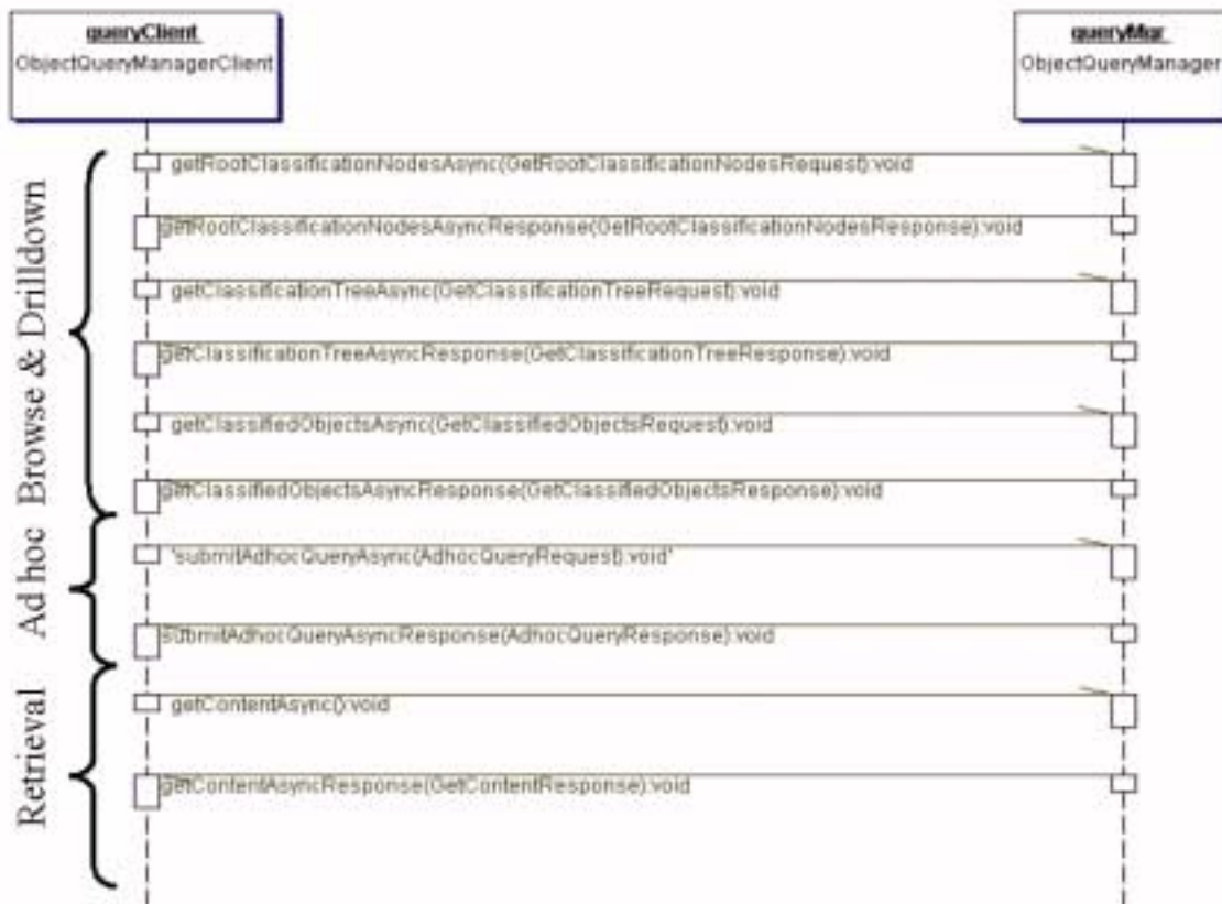
Figure 20: Typical Query and Retrieval Sequence
