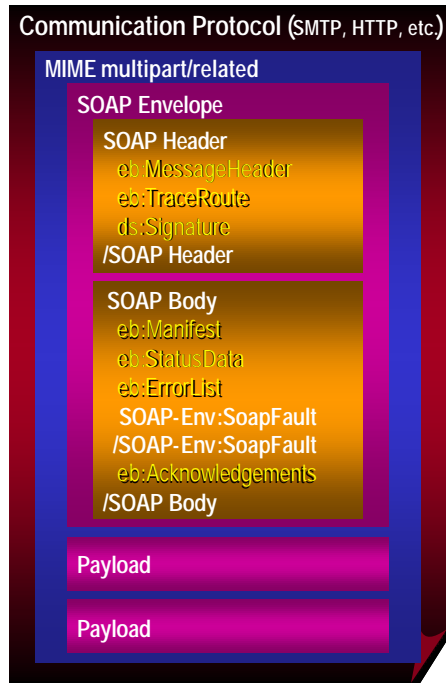
Figure 7 ebXML message structure
